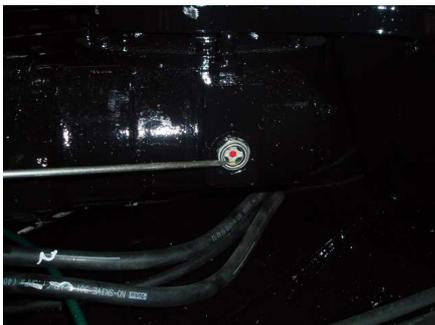
Figure 4.11 top up gear oil if necessary
