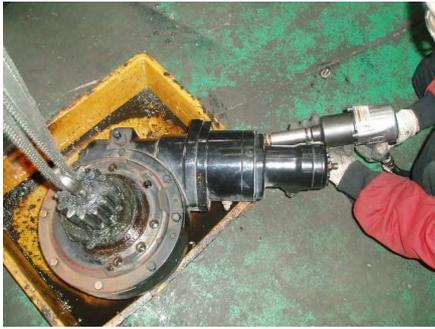
Figure 4.12 remove hydraulic motor
