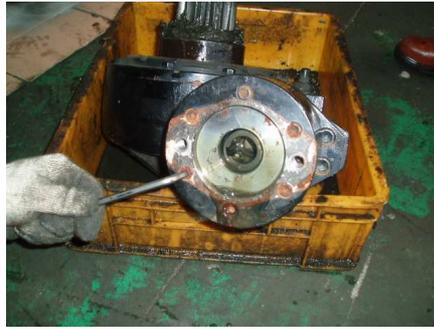
Figure 4.13 remove bolts for hydraulic brake cover
