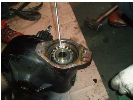
Figure 4.16 remove cogwheel washer
