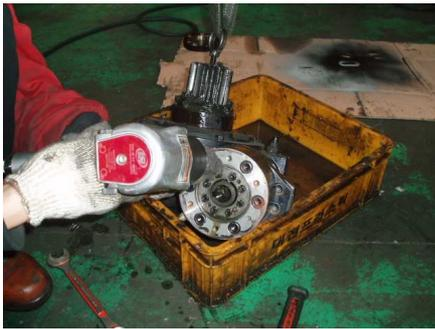
Figure 4.14 remove hydraulic brake
