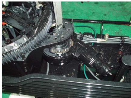
Figure 4.6 remove swing reducer
