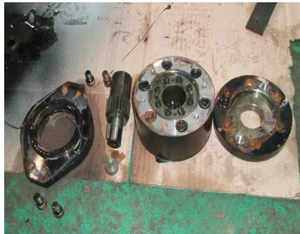
Figure 4.15 components of hydraulic brake
