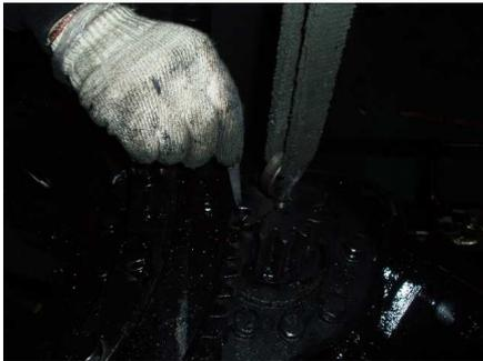
Figure 4.9 adjust backlash to 0.05-0.1mm
