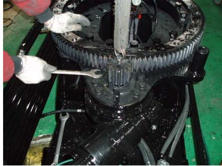
Figure 4.8 tighten bolts
