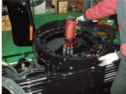
Figure 4.2 remove turntable bearing cover
