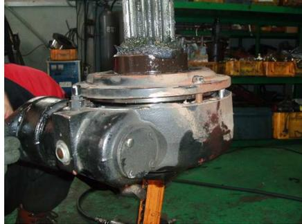
Figure 4.19 remove casing by screwing the bolts for removal
