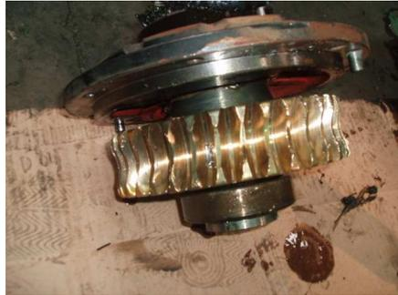
Figure 4.21 housing with gear shaft and worm wheel
