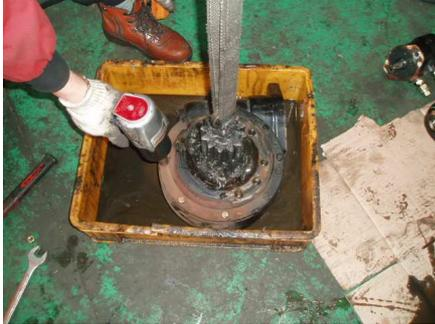
Figure 4.18 unscrew bolts for casing
