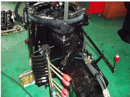
Figure 4.5 remove swing reducer
