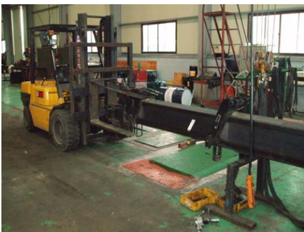
Figure 1.17 removal of 4 th to 6 th boom
