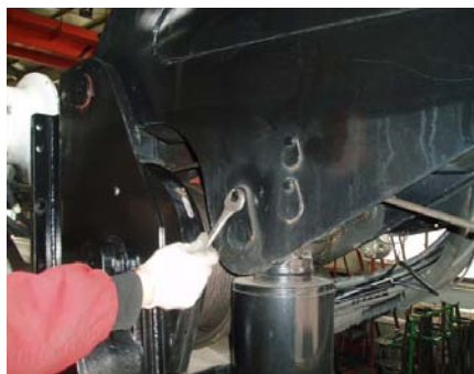
Figure 1.6 removal of derrick cylinder pin
