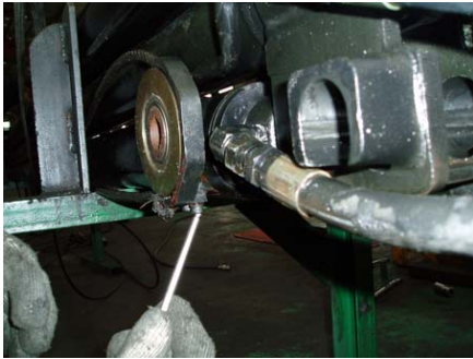
Figure 1.32 removal of wire rope
