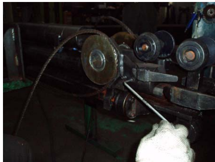
Figure 1.35 removal of wire rope
