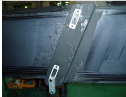
Figure 1.27 removal of side pads
