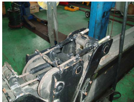
Figure 1.16 removal of 4 th to 6 th boom
