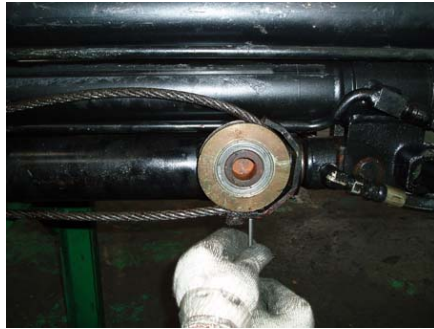
Figure 1.33 removal of wire rope
