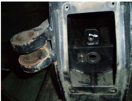
Figure 1.20 removal of the bolt
